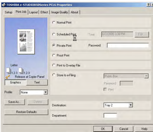
Things get interesting on the second tab of the driver (in this case, PCL), with Normal, Scheduled, Private, Proof, Print to Overlay, and Store to e-Filing selections. Also, users can save printing profiles from here while specifying output tray destination and department code (for print audit uses).
