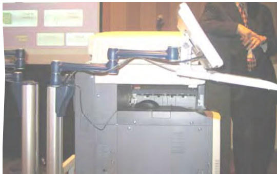
Above: ScanStation touchscreen interface Below: Swivel-mounted stand
