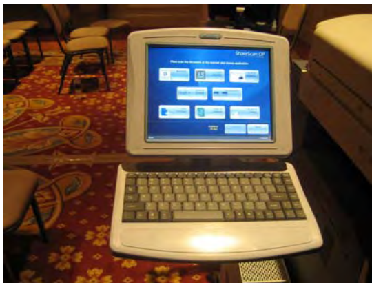
Above: ScanStation touchscreen interface Below: Swivel-mounted stand
