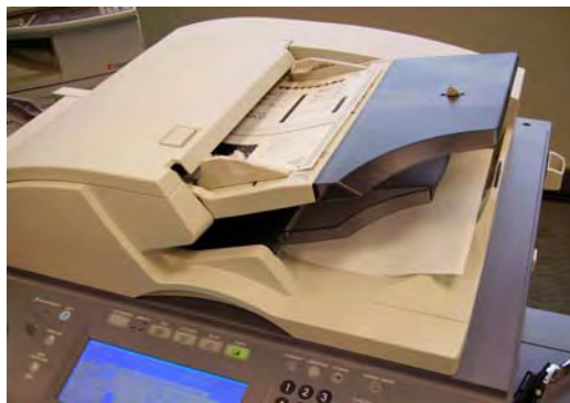
The automatic document feeder of the e-STUDIO 850 is convenient to use—and fast, scanning up to 71 ppm at 600 dpi resolution.
